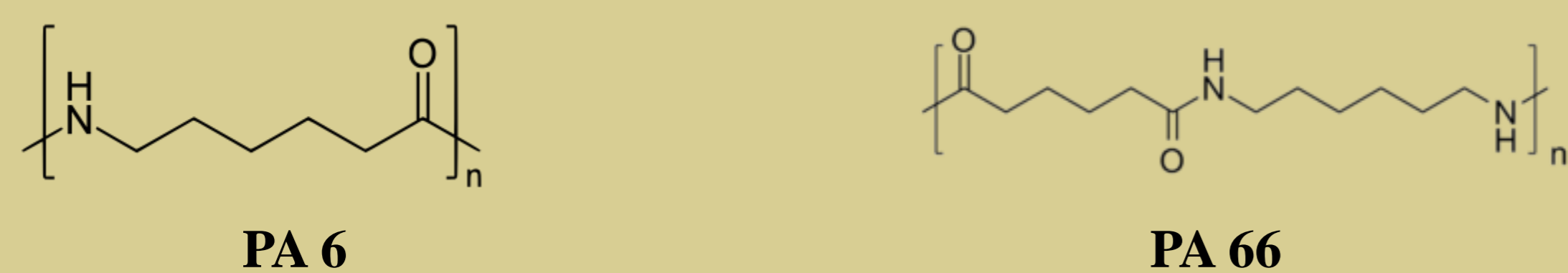
Figure 1. PA 6 and PA66 structure
