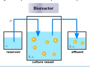
Bioreactors are devices in which cell cultures can be grown. In continuous fermentation, fresh medium is supplied continuously to the tank while used medium with toxic metabolites, consumed nutrients and cells are removed simultaneously.
