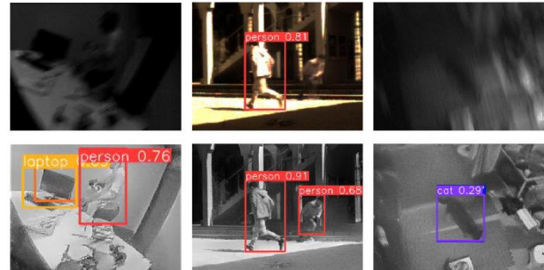
Figure 1. Comparison of detection on conventional frames (top) and reconstructed frames from event data (bottom).
