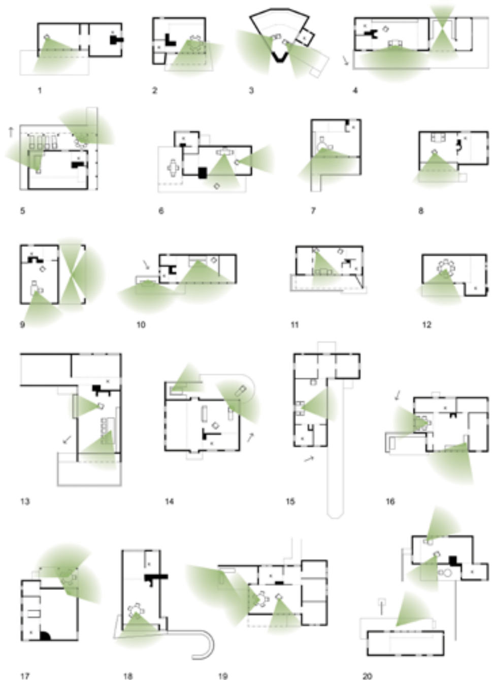
Figure 7. Views from the interior spaces framed by the huts' main openings. The black arrows point towards the south, as indicated in the original drawings. Hearths are represented through black hatches and the letter "K" means 'kitchen'. Interior partitions are also represented, and the different line weights imply the different degrees of disengagement of the spaces in relation to the main space.
